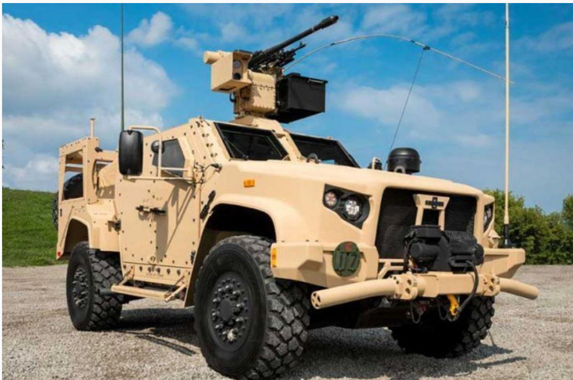
PHOTO: Oshkosh Joint Light Tactical Vehicle (JLTV) fitted with the EOS R400 Dual RWS with M230LF 30mm cannon and 7.62mm machine gun. (EOS)
